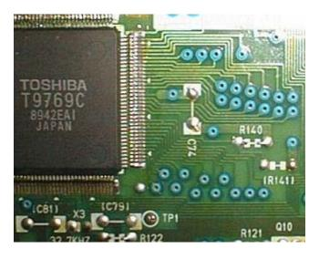
R140 and R141 on the back side of Panasonic FS A1WSX PCB
